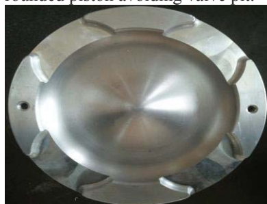
Fig 6 The result of milling
